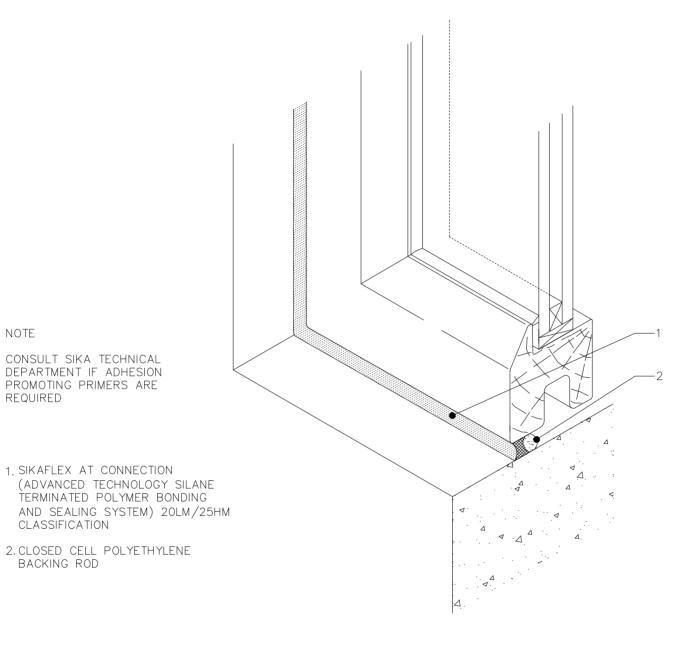
SIKA LIMITED SIKAFLEX AT CONNECTION ADVANCED TECHNOLOGY SILANE TERMINATED POLYMER BONDING AND SEALING SYSTEM 20LM/25HM CLASSIFICATION FULL SEAL AROUND WINDOW SB016
